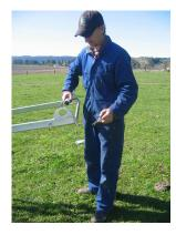
**Step 3 Insert Wrangler Back Leg Bar** into *Side Bars* and secure with R Clip.
