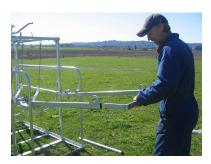
Step 2 Insert Locking Bar into end of *Side Bars*. Secure each side with *Shaft Locking Pin*. Note: If holes don't line up well try flipping *Locking Bal*
